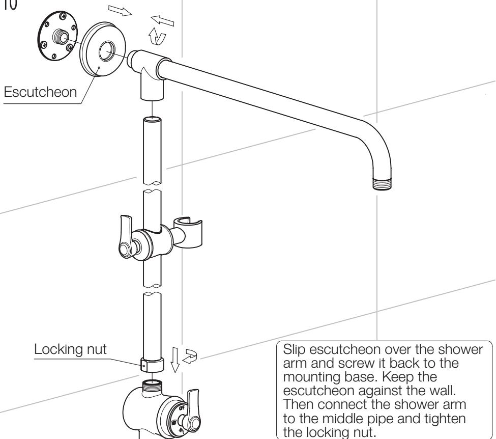
Slip escutcheon over the shower arm and screw it back to the mounting base. Keep the escutcheon against the wall. Then connect the shower arm to the middle pipe and tighten the locking nut.
