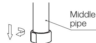
Remove the cap from the middle pipe, and be careful not to drop the rubber washer. Connect the middle pipe to the mixer body.
