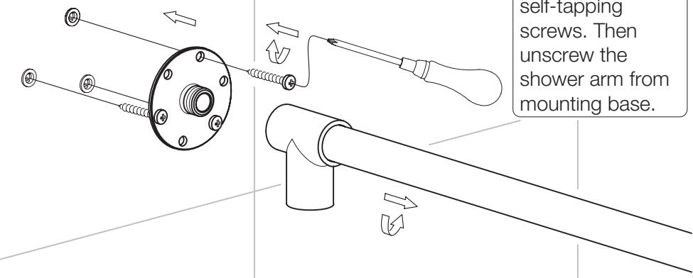
Fix mounting base to the wall with self-tapping screws. Then unscrew the shower arm from mounting base.
