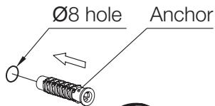
Remove shower arm and middle pipe. To prevent sand or other debris from falling onto the product during drilling, please cover the mixer body with a cloth bag. Drill three Ø8 holes at the marked positions and insert anchors.
