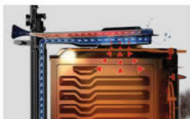
Dual cooling air flue
