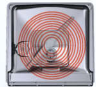
Conventional spray arms create circular washing zone
