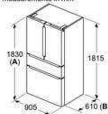
A: Front is adjustable from 1830 to 1847, with front levelling feet fully extended.
