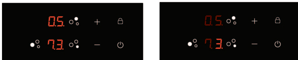
Fig. 6.: Selected cookset 3. Heater selection finished
