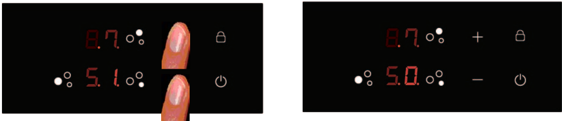
Fig. 14.: Switching off a heater touching the [+] and [-] keys
