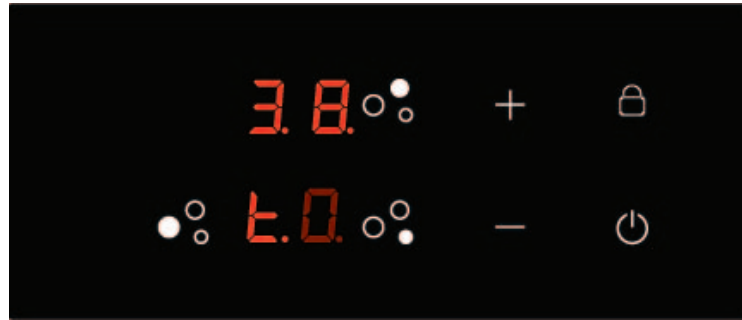
Fig. 23.: Selecting the remaining time for a heater.
